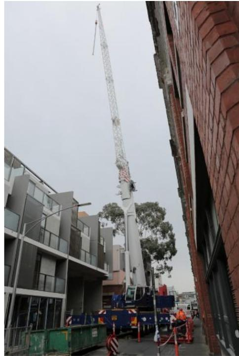
The Tadano model ATF220G-5 is a 5 axle crane with ratings of 12t per axle, has full hydraulic suspension, 85 kph road speed and 69% grade ability. Using the single cylinder telescoping system, the six-section boom extends to 68m. Additional boom extensions are available from 13.2m to 37.2m. This is a crane designed to be mobile yet capable of handling the big lifting jobs.
